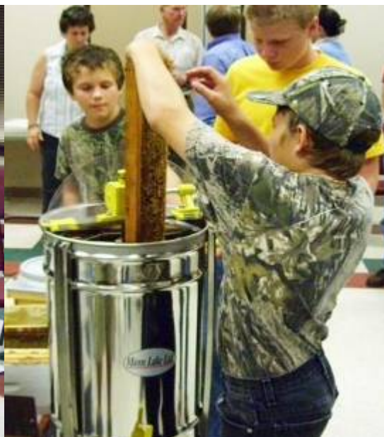
Michael Tutor loading frame into the extractor
